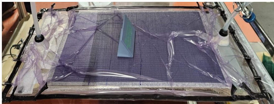
Figure 2 Vacuum infusion process
