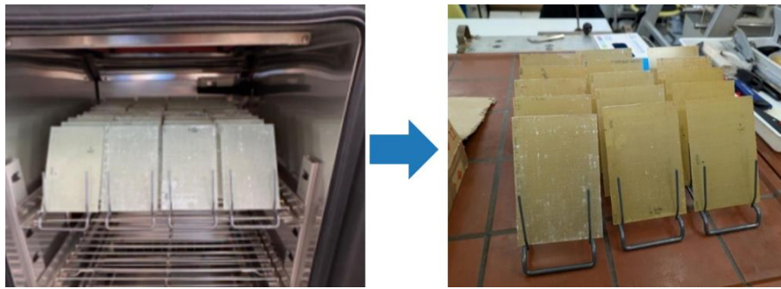
Figure 3 Aging of the sample plates in the climate chamber
